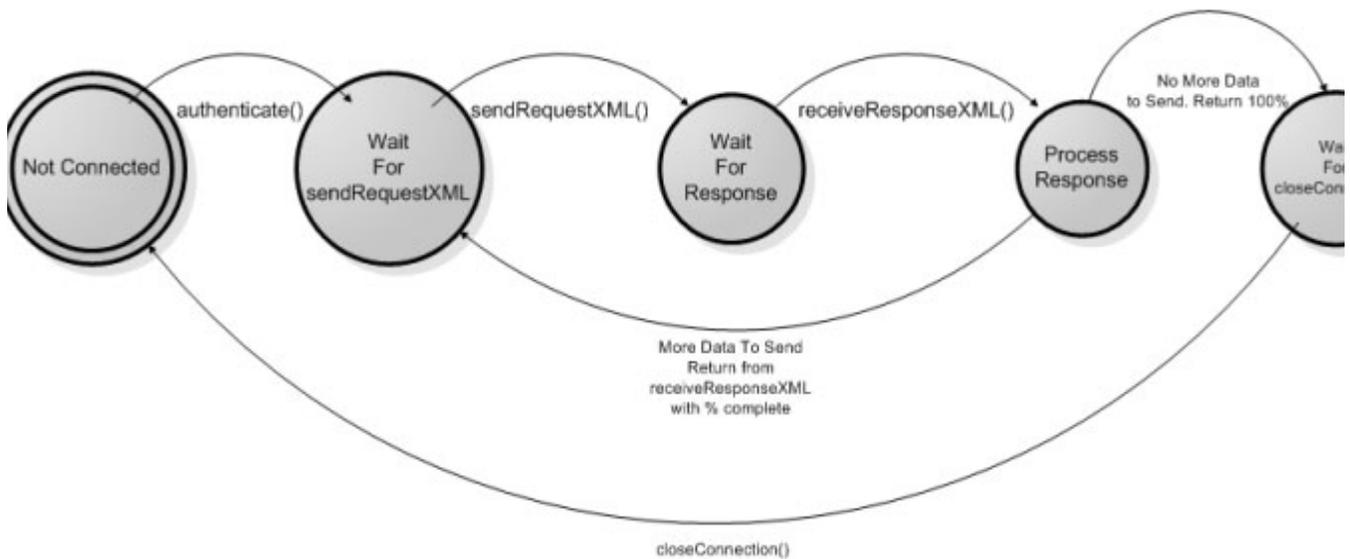
Figure 5-1 The Web Connector Service State Model
